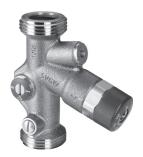
The Viega ProPress Automatic Recirculation Regulating Valve provides automatic balancing of domestic hot water recirculation return lines. Balancing based on hot water return temperature allows the recirculation system to run more efficiently with smaller pipes and circulators.
