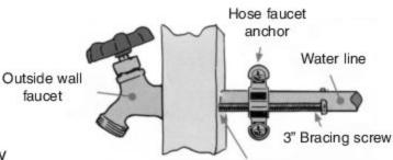
Bracing screws may dig into the wood or masonry material
