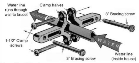
Loosely assemble clamp halves around the hose faucet water line on the inside of the wall using the shorter (11/2") screws.
