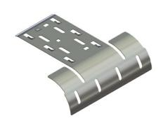
The Basic Dropout (BDO) smooths the transition of cabling dropping out of wire mesh tray. These dropouts snap into place without hardware and reduce the strain of cables as they exit or enter the tray. It mounts at the end of the wire basket cable tray parallel or perpendicular to the tray bottom.
