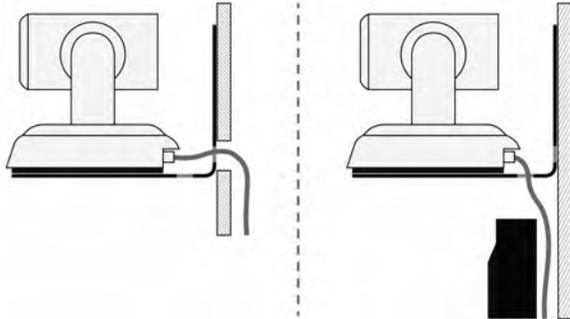
6. Attach the camera to the mount using the 1/4"-20 x .375 mounting screw supplied with the camera.
