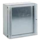
Clear molded polycarbonate window has a 31.8-mm (1.25-in.) clear space between enclosure front opening and window surface. Space also accommodates equipment mounted on optional front plate. Window kit is hinged on left side with a 140-degree door opening and a quarter-turn slotted latch. Includes mounting hardware for window and optional front plate. Die-cast backing plate has a black polyester powder finish. This kit can be used as an accessory window kit on other Hoffman enclosures.
