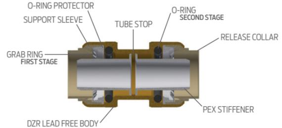
Only when the pipe has passed through the o-ring and reaches the tube stop is a secure joint created. The SharkBite fittings can only be used with pipe/tubing certified to the following specifications:
