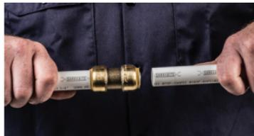
Once the pipe end is cut square and clean, use the SharkBite Depth Debur Gauge (sold separately) and a permanent marker to mark the insert depth on the outside of the pipe. This mark is used to ensure that the joint is assembled correctly. To assemble correctly, the pipe needs to be pushed into the fitting until it meets the tube stop. Follow these three steps to insert the pipe into the fitting.
