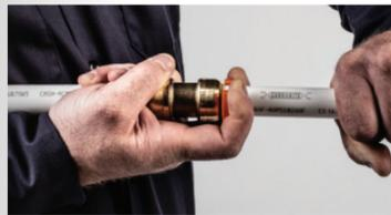
1. Place the SharkBite disconnect clip around the pipe with the non-branded face against the release collar. If using the SharkBite disconnect tongs, place the teeth around the fitting assembly. The fork end with the SharkBite brand logo should be positioned around the pipe and the other end around the neck of the fitting.
