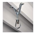
The 115M Standard Duty Loop Hanger is ideal for suspending stationary, non-insulated pipe lines, including CPVC pipes, in fire sprinkler systems. A knurled insert nut helps simplify vertical adjustments and flared edges on the base (1/2" to 4" sizes) help protect pipes from coming into contact with any sharp edges of the hanger.
