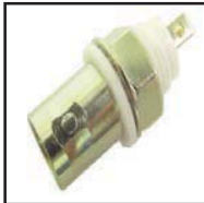
75-514 BNC Female, isolated ground from chassis. Length is 1.06". Mounts in .37" chassis hole. Bushing length .38".
