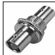
75-552 BNC feed thru double Female panel mount. Mounts in .5" D hole. Overall length is 1.28". Bushing length .33". 75-696 75 ohm version
