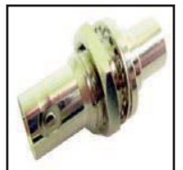
75-521 Panel feed thru connector. BNC Female to RCA Female. Bushing dia.: .487". Bushing length: .33". Overall length is 1.29". Mounts in .5" hole. 75 ohm. 75-521-50 50 Ohm version
