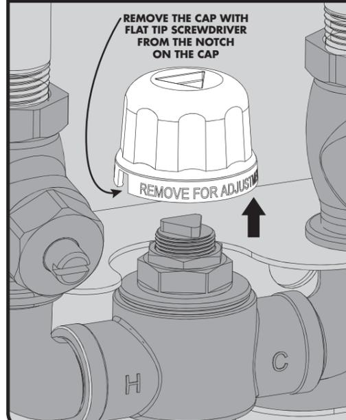
This Mixing Valve has been set at the factory to deliver 85 °F outlet flow. High temperature limit is set to 94 °F by design. Should the Valve require adjustment, or an application require a different set temperature, proceed as follows:
