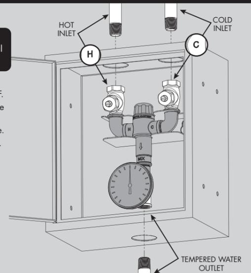
**WARNING:** The Valve will not function in the way it is intended to if Cold water supply pipe is connected to "H" Inlet on Valve and Hot water supply pipe is connected to "C" inlet on Valve.
