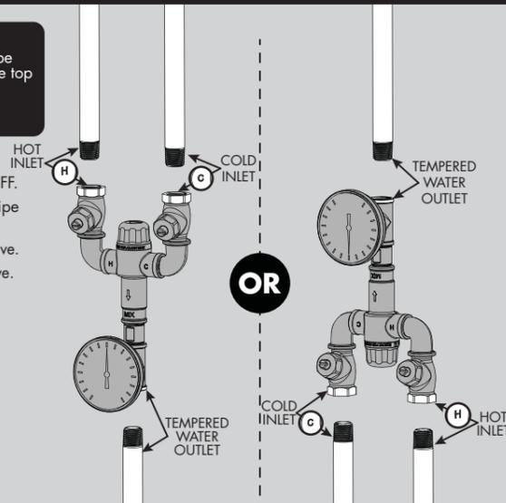
**WARNING:** The Valve will not function in the way it is intended to if Cold water supply pipe is connected to "H" Inlet on Valve and Hot water supply pipe is connected to "C" inlet on Valve.
