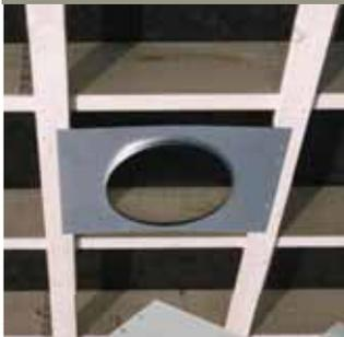
Model RCF Designed for new construction. Our RCF flashing can be fastened to rough framing. It has a 3/8" lip that drops below the ceiling, requiring dry wall installers to cut the hole for you. RCF flanges are available for both 16" and 24" on center framing.
