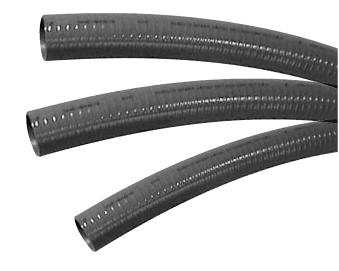
**Note**: Liquidtight flexible conduits, metallic and non-metallic, in contrast to rigid PVC conduit and electrical non-metallic tubing, does not have wire temperature limitations. Any temperature-rated wire (for example, 90° wire) can be used as long as the temperature conditions marked on the conduit are not exceeded. UL Listed conduits that are not marked are limited to a maximum temperature of 60° C wet or dry.
