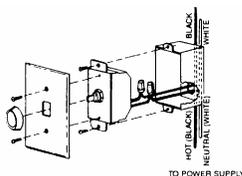
Figure 2 - Wiring
