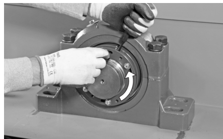
Figure 4 - Holding external nut and rotating internal nut using hex head bolt
