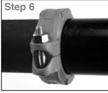
Assembly is completed 6 Assembly is compared to assure the coupling keys are fully engaged in the pipe grooves and the bolt pads are in firm even metal-to-metal contact on both sides of the coupling.
