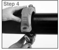
Housings Place the coupling housing halves over the gasket making sure the housing keys engage the grooves. Insert bolts and turn nuts finger tight.
