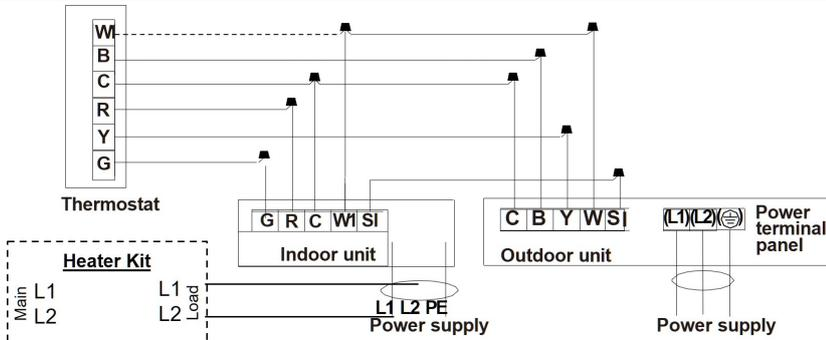
Note: When Heater Kit is installed, connect AHU power (White/Black pigtail) to load side of appropriate breaker to power AHU. For 15KW/20KW connect to "CB1" which is L1/L2 of the included wiring diagram.
