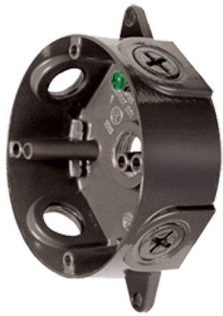
Die cast aluminum wiring box with ground screw, and two sturdy lugs for wall or ceiling mounting. Supplied with four color matched close-up plugs. Color: Black Weight: 0.5 lbs
