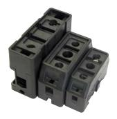
All 30, 60 and 100 A CUBEFuse holders dovetail together to create the desired number of poles. Each holder accepts CUBEFuse amp ratings up to its rating. E.g., the 60 amp holder will accept a CUBEFuse from 1 to 60 A.
