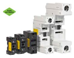
The Bussmann series CUBEFuse holder is a finger-safe modular system of single-pole 30, 60, 100, 200, 225 and 400 amp holders. All holders dovetailed together to create the desired number of poles for the application, including mixed amp ratings between the 30, 60 and 100 amp holders.
