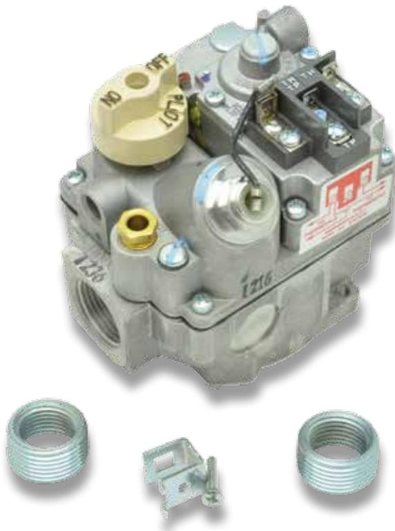
The Robertshaw® Unitrol® 7000 is Simply the Right Choice™ for gas cooking controls. The Unitrol 7000 models combine a manual main and pilot gas valve, a separate automatic safety pilot valve, pilot adjustment valve, and a diaphragm valve. The regulated models also feature “straight line” gas pressure regulation.
