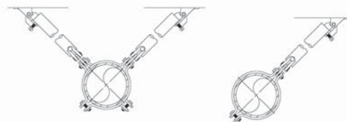
4-Way Riser Brace (Plan view)
