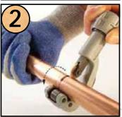
Cut COPPER, CPVC or PEX using a quality Tuber or Pipe Cutter with a sharp blade.
