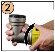
Rotate Shark Shifter De-Mount Tool clockwise to locate on lugs, rotate a further 1/2" to disconnect.
