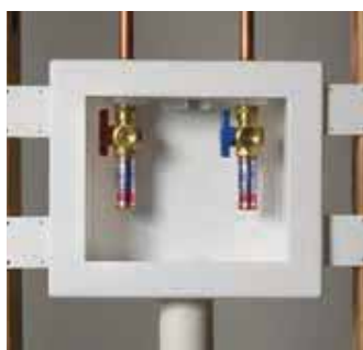
Top mount 1/4 turn hammer arrestor valves with copper connections & center drain.
