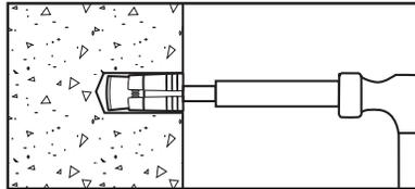
Insert the anchor into the hole. Position the setting tool in the anchor.
