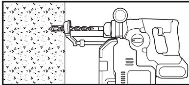
Drill a hole into the base material to the required embedment depth. The tolerances of the drill bit used must meet the requirements of ANSI Standard B212.15.
