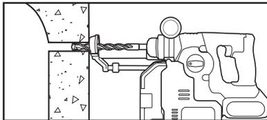
In hollow base materials, drill through into the cell or void. The tolerances of the drill bit used must meet the requirements of ANSI Standard B212.15.
