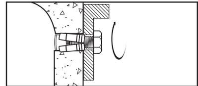
Position fixture, insert bolt and tighten. The bolt should engage a minimum of 2/3 of the anchor threads. The anchor can also be expanded using a Hollow-Set Tool. (If Hollow-Set Tool is used, thread anchor onto tool prior to tapping into anchor hole. When flush with surface, turn tool clockwise to tighten. Release tool from set anchor by turning counterclockwise. Fixture can then be attached).
