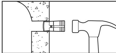
Do not expand the anchor prior to installation. Insert cone end and tap flush to surface.
