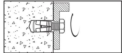
Be sure the anchor is at the required embedment depth, so that anchor threads do not protrude above the surface of the base material. Position the fixture, insert bolt or threaded rod and tighten.
