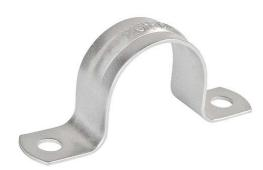
These two hole rigid and IMC conduit straps are used to mount 3" rigid or IMC conduits where higher load bearing supports are needed. Garvin Industries' two screw holes allow the installer to secure pipes on walls and ceilings. They also prevent accidental pullout in high traffic areas.
