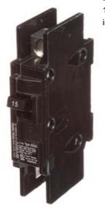
Siemens Low Voltage Molded Case Circuit Breakers General Purpose MCCBs are Circuit Protection Molded Case Circuit Breakers. 1-Pole circuit breaker type BQXD. Rated 120V (015A) (AIR 10 kA). Special features: DIN Rail mounted, Line and load side lugs included..
