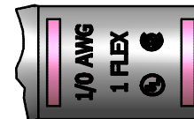
DETAIL C BOTTOM INK MARKING INK COLOR: PINK PER SPEC #: F921
