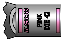
DETAIL A TOP INK MARKING INK COLOR: PINK PER SPEC #: F921
