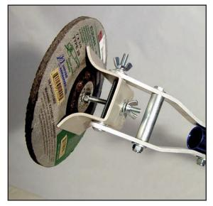
2. Place the large washer (006) and the small washer (007) on the bolt. Secure with the wing nut (008).
