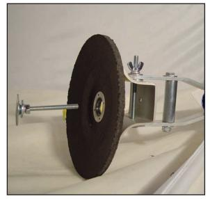
1. Thread the bolt with dimpled washer (002), two washers (003), 1 small lock washer (004), and the nut (005) through the hole in the bottom of the disc and through the hole in the assembly bracket.
