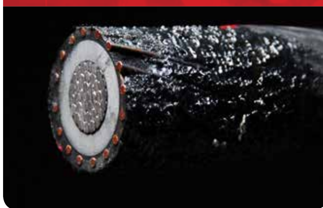
Unprotected Cable After Test
