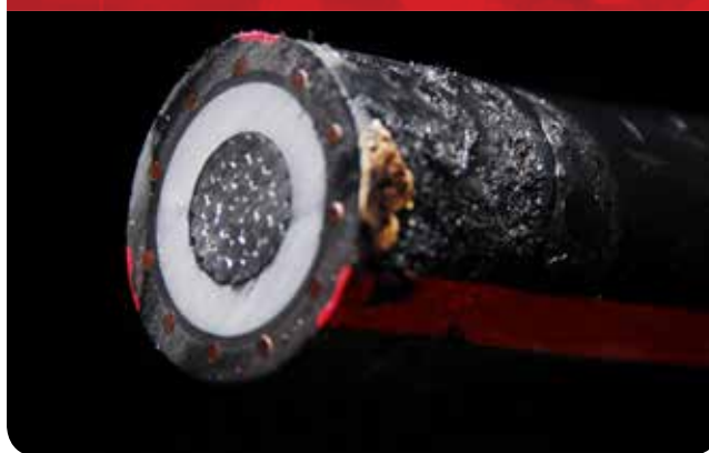
Cable Protected with Scotch® Tape 77 After Test
