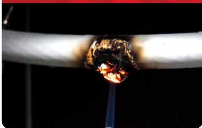
Cable Protected with Scotch® Tape 77 During Test
