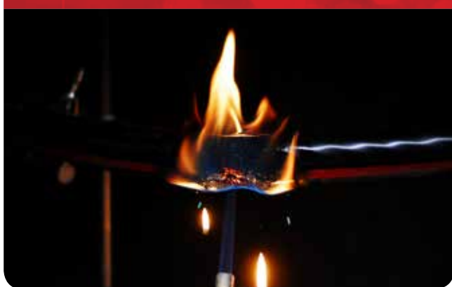
Unprotected Cable During Test
